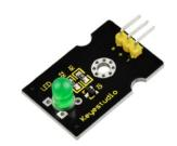
This is a green LED module. The main function is to control a plugin LED on and off. When connecting to ARDUINO, after programming, it will emit green light color. The pin pitch of 3Pin is 2.54mm
